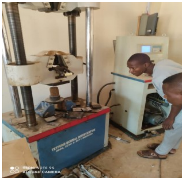
Plate 9: Determining compressive strength using universal testing machine
