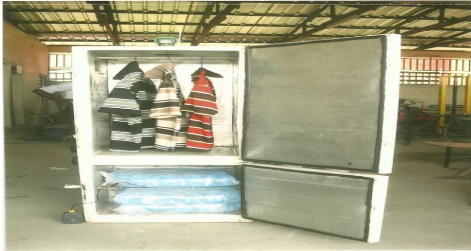
Patented photograph of Integrated Tetrafluoroethane (R-134a) Refrigerator-Dryer
