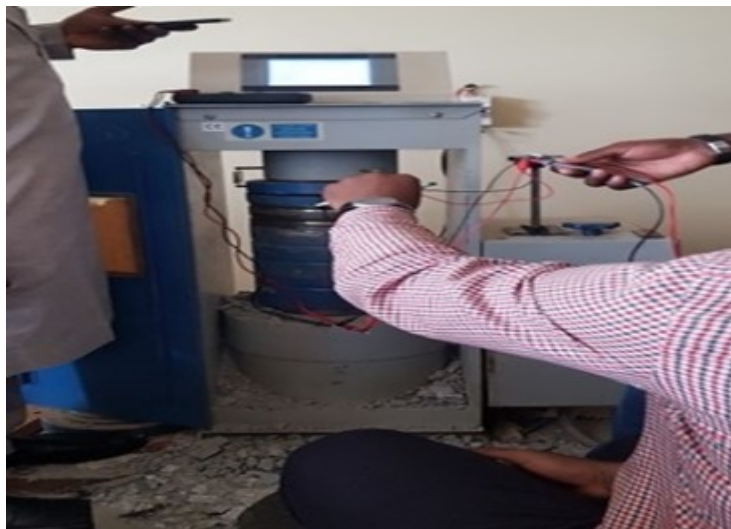
Figure 4: Mechanical testing using an Automatic Compression Machine (ACM) to apply pressure to the stacked piezoelectric tiles
