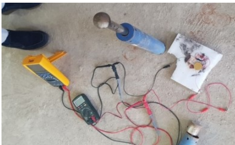
Figure 5: Mechanical testing using a 2.5kg proctor compaction rammer to apply pressure to the piezoelectric tiles.
